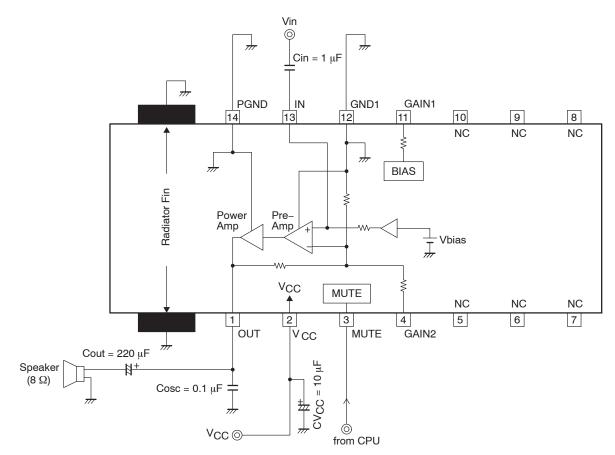
Figure 3. Block Diagram and Sample Application Circuit
